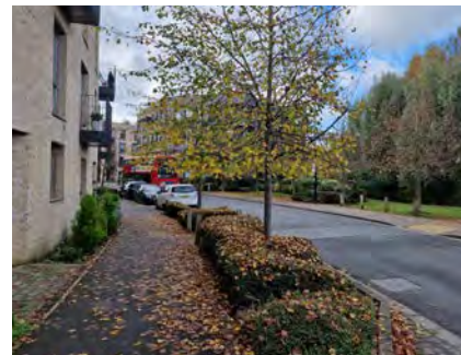
Evergreen shrub species planted within verges to prevent verge parking
