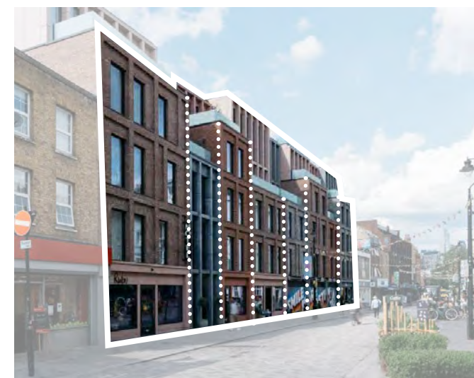
Subdividing the frontage of a single building to match the prevailing grain and rhythm of a High Street (Lower Marsh, Waterloo)
